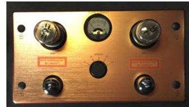
Bias Setting for Power Tubes
